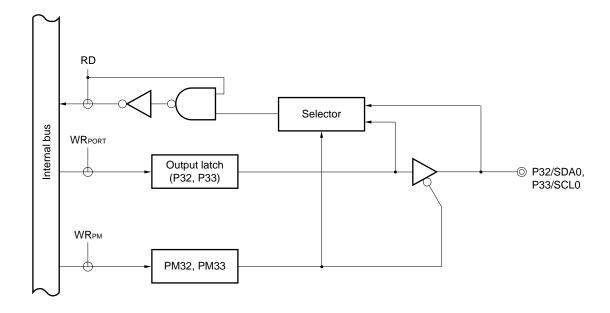
PM: Port mode register RD: Port 3 read signal WR: Port 3 write signal
