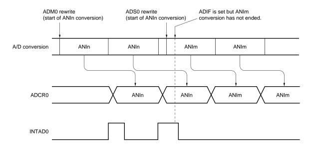
Figure 14-11. A/D Conversion End Interrupt Request Generation Timing
