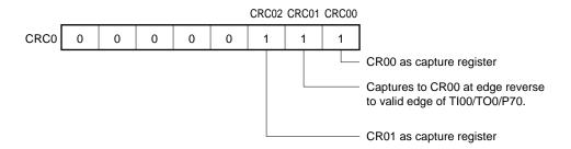
**Remark** 0/1: Setting 0 or 1 allows another function to be used simultaneously with pulse width measurement. See the description of the respective control registers for details.
