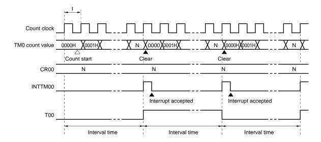
**Remark** Interval time =  $(N + 1) \times t$ : N = 00H to FFH
