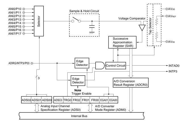
Figure 13-1. 8-Bit A/D Converter Block Diagram
