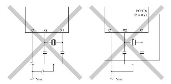
**Remark** When using a subsystem clock, replace X1 and X2 with XT1 and XT2, respectively. Further, insert resistors in series on the side of XT2.
