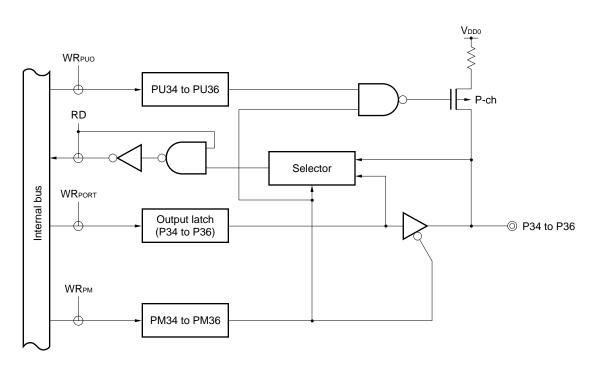
Figure 6-9. P34 to P36 Configurations (μPD780024Y, 780034Y Subseries)
