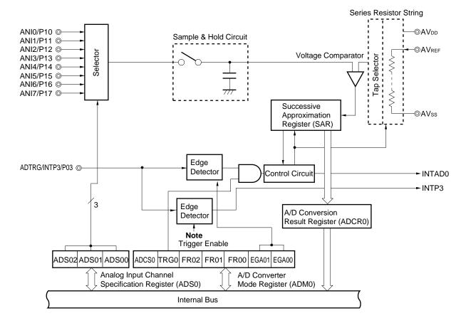
Figure 14-1. 10-Bit A/D Converter Block Diagram
