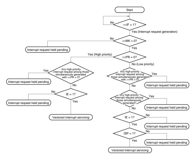
Figure 19-10. Interrupt Request Acknowledge Processing Algorithm
