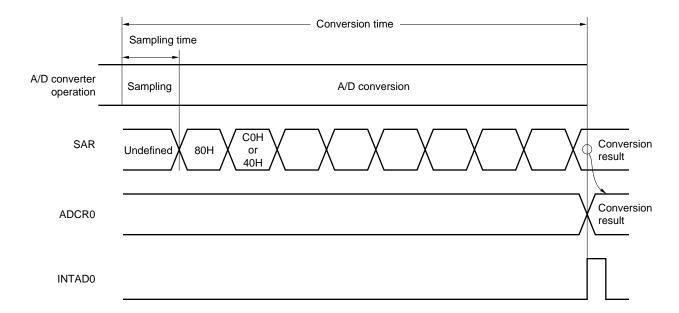
Figure 13-5. Basic Operation of 8-Bit A/D Converter
