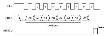
**Note** INTIIC0 is not issued if data other than a local address or extension code is received during slave device operation.
