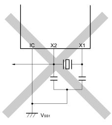
**Remark** When using a subsystem clock, replace X1 and X2 with XT1 and XT2, respectively. Also, insert resistors in series on the XT2 side.
