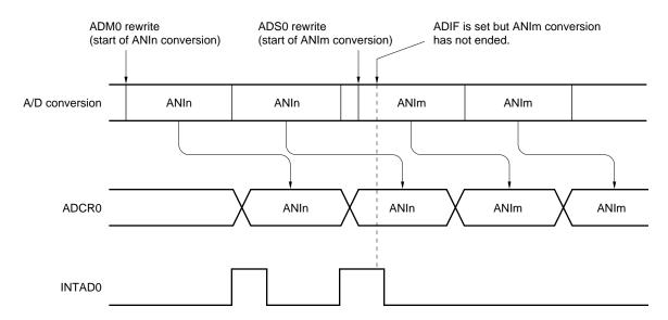
Figure 13-11. A/D Conversion End Interrupt Request Generation Timing
