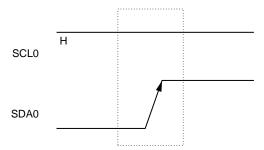
A stop condition is generated when bit 0 (SPT0) of the IIC control register (IICC0) is set (to "1"). When the stop condition is detected, bit 0 (SPD0) of the IIC status register (IICS0) is set (to "1") and INTIIC0 is generated when bit 4 (SPIE0) of IICC0 is set (to "1").
