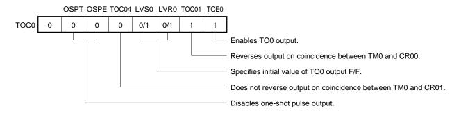
**Remark** 0/1: Setting 0 or 1 allows another function to be used simultaneously with square-wave output. See Figures 8-2, 8-3, and 8-4.
