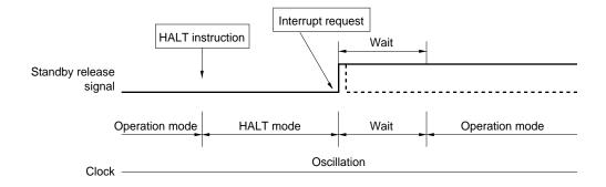
**Remarks 1.** The broken line indicates the case when the interrupt request which has cleared the standby mode is acknowledged.
