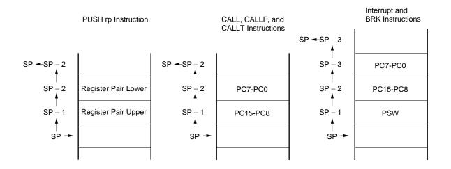
Figure 5-15. Data to be Restored from Stack Memory
