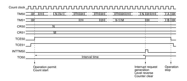
Figure 9-12. 16-Bit Resolution Cascade Connection Mode
