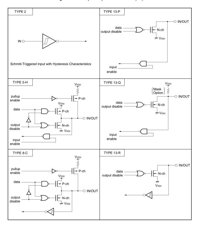
Figure 3-1 Pin Input/Output Circuit of List (1/2)
