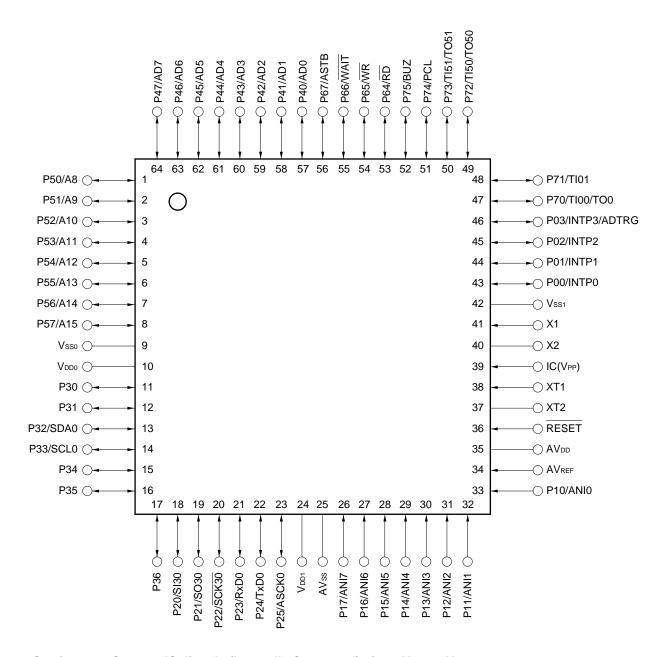
Cautions 1. Connect IC directly (Internally Connected) pin to Vsso or Vsso.
