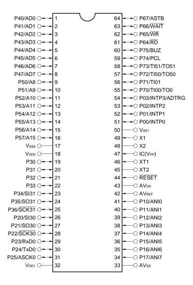
Cautions 1. Connect directly IC (Internally Connected) pin to Vsso or Vss1.
