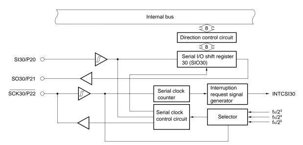
Figure 17-1. Serial Interface (SIO30) Block Diagram
