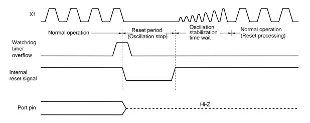
Figure 22-4. Timing of Reset in STOP Mode by RESET Input
