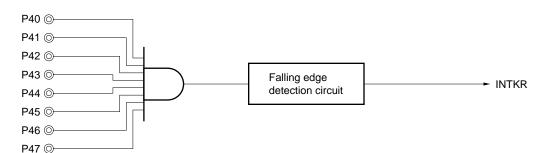
Figure 6-11. Falling Edge Detection Circuit Block Diagram
