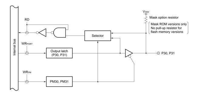
PM: Port mode register RD: Port 3 read signal WR: Port 3 write signal
