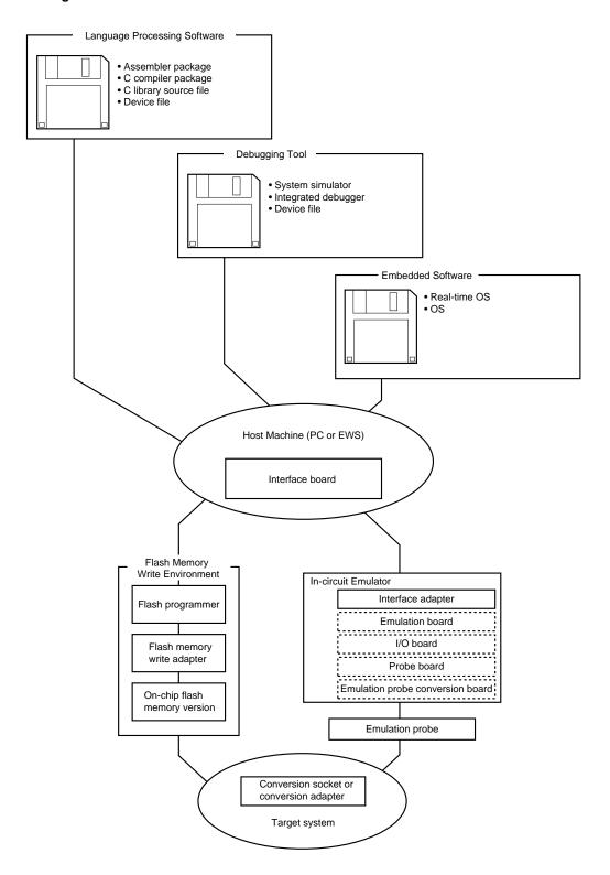
**Remark** Items in broken line boxes differ according to the development environment. Refer to **B.3.1. Hardware**.
