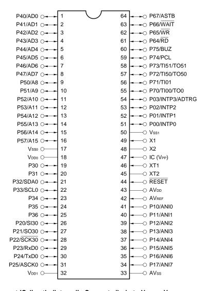
Cautions 1. Connect IC directly (Internally Connected) pin to Vsso or Vsso.
