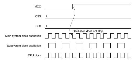
Figure 7-7. Main System Clock Stop Function (2/2)
