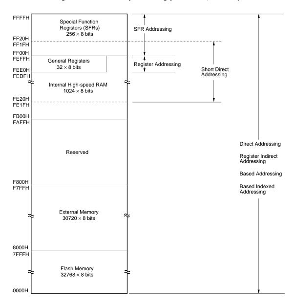
Figure 5-10. Data Memory Addressing ( $\mu$ PD78F0034, 78F0034Y)
