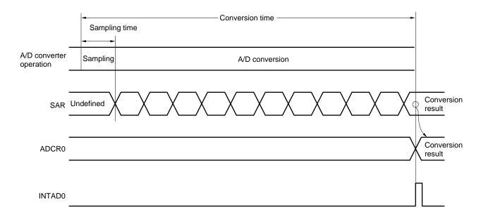
Figure 14-5. Basic Operation of 10-Bit A/D Converter
