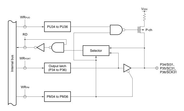
Figure 6-6. P34 to P36 Configurations ( $\mu$ PD780024, 780034 Subseries)
