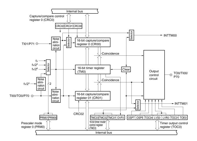
Figure 8-1. 16-Bit Timer/Event Counter Block Diagram
