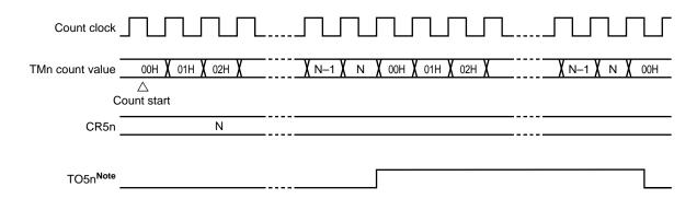
**Note** TO5n output initial value can be set by bits 2 and 3 (LVR5n, LVS5n) of the 8-bit timer mode control register 5n (TMC5n)
