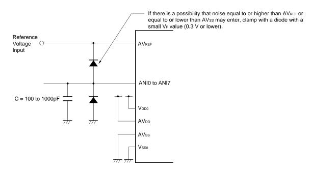
Figure 14-10. Analog Input Pin Connector
