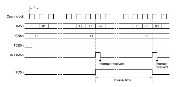
Figure 9-7. Interval Timer Operation Timings (3/3)
