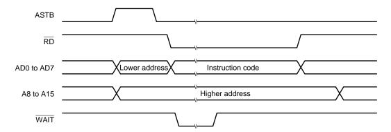
Figure 20-5. External Memory Read Timing
