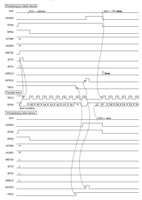
Figure 18-21. Example of Slave to Master Communication (when 9-clock Wait Is Selected for Both Master and Slave) (2/3)
