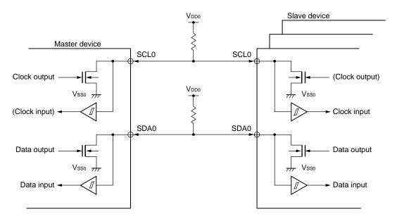
Figure 18-6. Pin Configuration Diagram
