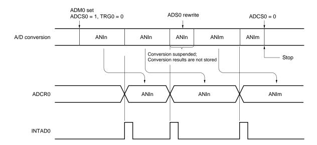
Figure 13-8. A/D Conversion by Software Start
