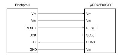
Figure 23-6. Flashpro II Connection Using Pseudo 3-wire Serial I/O
