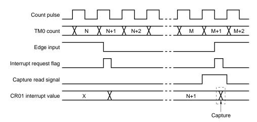
Figure 8-30. Capture Register Data Retention Timing
