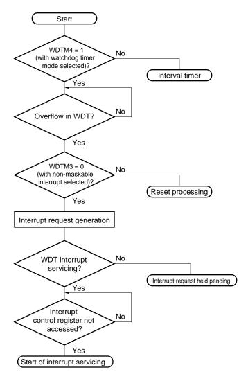
Figure 19-7. Non-Maskable Interrupt Request Generation to Acknowledge Flowchart
