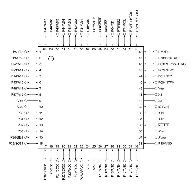
Cautions 1. Connect directly IC (Internally Connected) pin to Vsso or Vsso.
