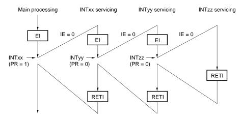
During servicing of interrupt INTxx, two interrupt requests, INTyy and INTzz, are acknowledged, and multiple interrupt servicing takes place. Before each interrupt request is acknowledged, the EI instruction must always be issued to enable interrupt request acknowledge.
