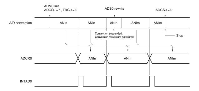
Figure 14-8. A/D Conversion by Software Start
