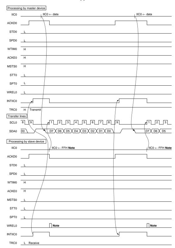
Figure 18-20. Example of Master to Slave Communication (when 9-clock Wait Is Selected for Both Master and Slave) (3/3)
