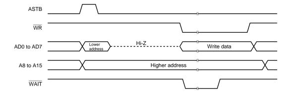
Figure 20-7. External Memory Read Modify Write Timing
