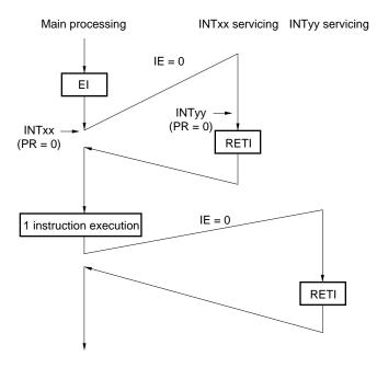
Interrupt is not enabled during servicing of interrupt INTxx (EI instruction is not issued), therefore, interrupt request INTyy is not acknowledged and multiple interrupt servicing does not take place. The INTyy interrupt request is held pending, and is acknowledged following execution of one main processing instruction.
