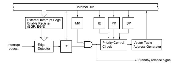
Figure 19-1. Basic Configuration of Interrupt Function (2/2)
