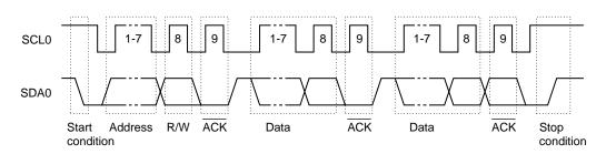
Figure 18-7. I<sup>2</sup>C Bus's Serial Data Transfer Timing
