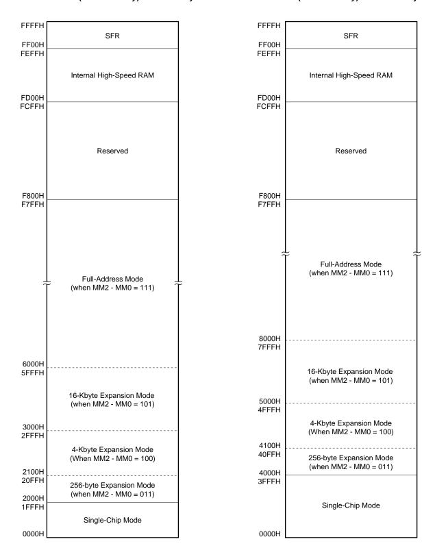
Figure 20-1. Memory Map when Using External Device Function (2/2)
