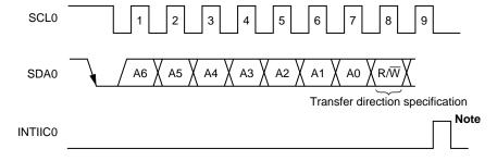
**Note** INTIIC0 is not issued if data other than a local address or extension code is received during slave device operation.
