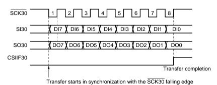
Figure 17-3. Timing of 3-Wire Serial I/O Mode
