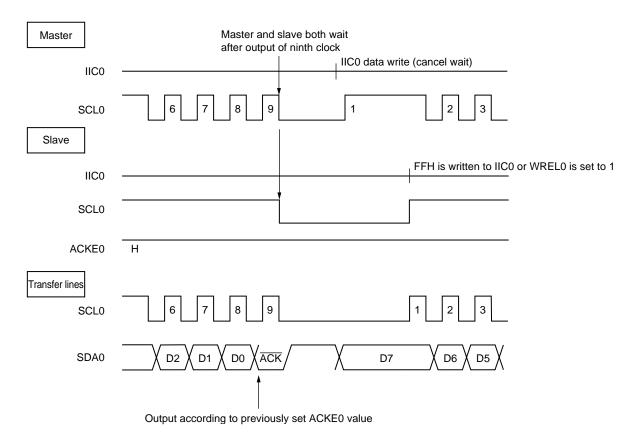
Remarks ACKE0: Bit 2 of IIC control register (IICC0)
