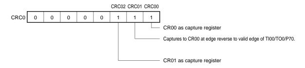
**Remark** 0/1: Setting 0 or 1 allows another function to be used simultaneously with pulse width measurement. See Figures 8-2 and 8-3.
