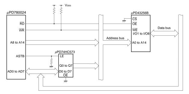
Figure 20-8. Connection Example of  $\mu$ PD780024 and Memory
